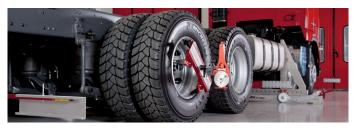
JOSAM laser AM can easily be configured to measure chassis frames. This is possible with additional frame gauges, a supplementary software or special report sheets. A frame check is part of every alignment procedure.
