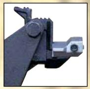
Quick-fit aluminium protectors and permanent vertical plastic protectors on jaws help prevent accidental damage to aluminium rims.
